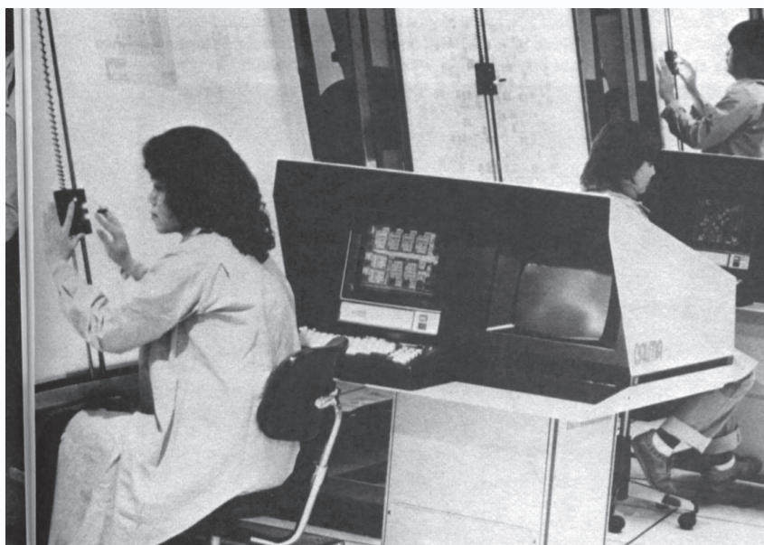
FIGURE 1: Digital design in the early 1980s using Calma stations. Figure courtesy of W. Harper.
